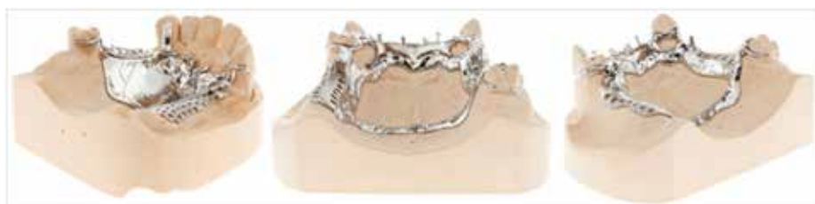
Figure 4. Completed CoCr Framework using DMLS produced by Dentwise. (By kind permission from 3D Systems Leuven.)
