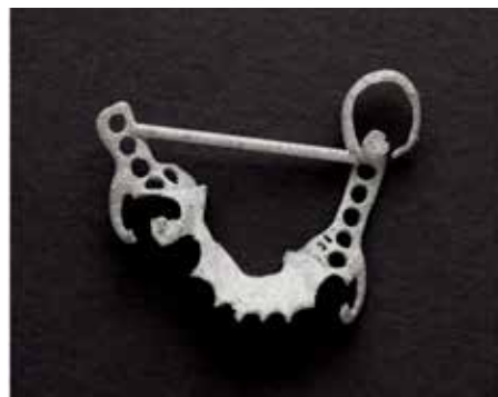
Figure 8. CoCr Framework once 3D printing complete.
