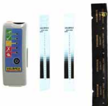
Figure 2. A commercially available system showing the device for reading the processed strips, two processed strips and a pre-exposed film strip in packet prior to processing.
