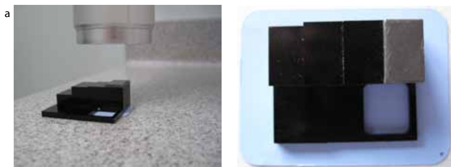
Figure 4. (a) Step test object placed on digital sensor used to assess grey levels. The step wedge images show different shades of grey depending on exposure.
