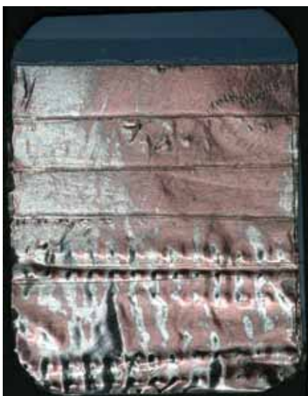
Figure 2. Home-made step wedge (test object) used for monitoring processing.
