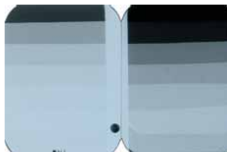
Figure 3. Appearances of radiograph of step wedge. Image on right would be the reference film and that on the left the possible image obtained if the developer was exhausted.
