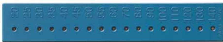
Figure 6. Sizing guides (Dentsply, Tulsa, USA) are an inexpensive method of confirming the size of the GP point selected. Simply insert the GP into the corresponding hole. If the GP point is smaller than the ISO size it will protrude beyond the guide and can be simply cut to length with a scalpel. If the point is too large select another point.
