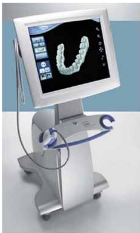
Figure 3. LAVA chairside intra-oral scanner (courtesy of 3M ESPE).
