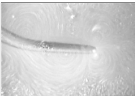
Figure 2. Acoustic streaming patterns, observed in water around an ultrasonic scaling tip, caused by the high frequency oscillations. (Adapted from Khambay and Walmsley. 2 )
