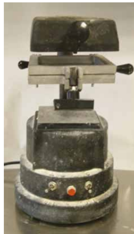
Figure 5. Vacuum thermoforming machine.
