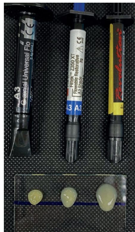
Figure 2. Different flowability after 60 seconds of three different conventional FCs by using the drip method.
