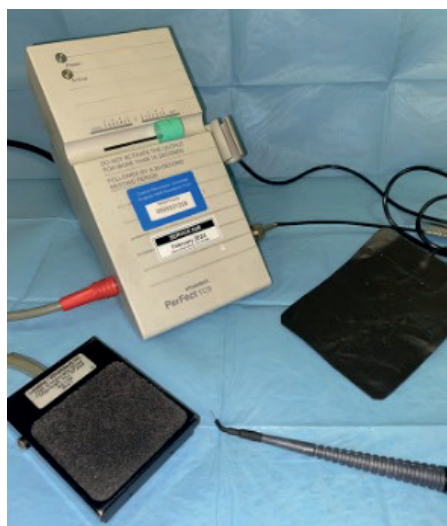
Figure 1. A standard electrosurgery unit with a current generator, handpiece, ground plate and foot control.
